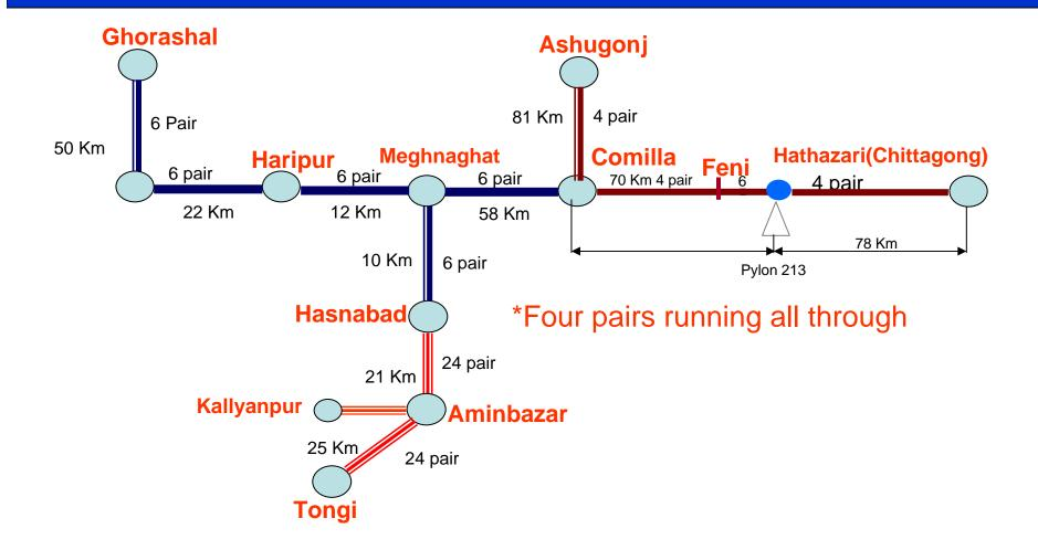
Under NLDC project about 1450 Km optical fiber will be installed on the existing transmission lines throughout the whole country by FY 2007.
