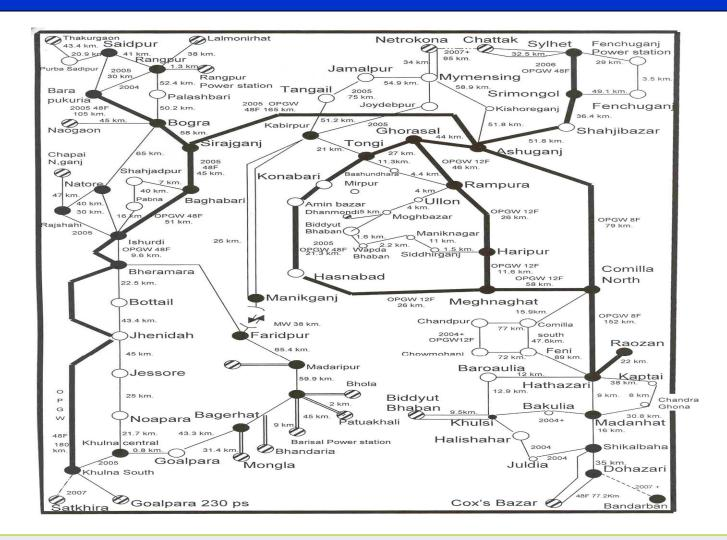
After completion of NLDC project most of the district towns of Bangladesh could be connected at Cox's Bazar with the optical submarine cable.
